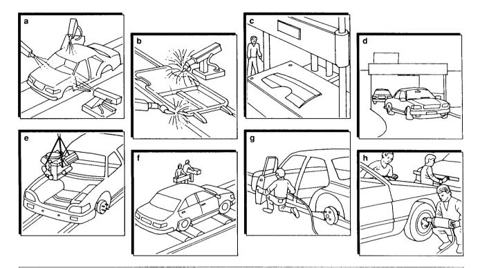
the finished car – test the car – despatch the body – paint the body panels – cut the components – fit the engine – put in the doors – add the panels – weld
